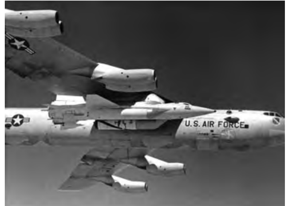
B-52 mother ship with X-15A-2. The latter mounted a dummy scramjet and carried external tanks as well as ablative thermal protection. (NASA)
